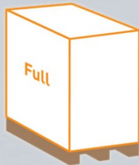
Full Pallet 1.2m x 1.2m x 2.44m high Maximum weight 1,250kg
