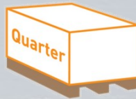
Quarter Pallet 1.2 x 1.2m x 1m high Maximum weight 250kg
